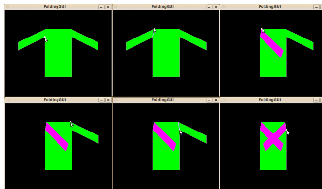
Fig. 10 An example sequence of user-specified folds. The user first clicks on the left arm-pit, then on the left shoulder to specify the first fold. The GUI then verifies that this is a valid g-fold for the chosen number of grippers. In this case it is, and it then shows the result after executing the g-fold (3rd image in the top row). Then the user specifies the next fold by two clicks, the program verifies whether it's a valid g-fold, and then shows the result after executing the g-fold.
