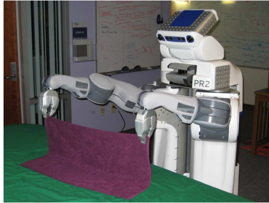
Fig. 8 The PR2 robotic platform (developed by Willow Garage) performing a g-fold on a towel.
