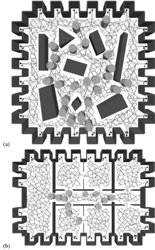
Fig. 3. Two environments and their roadmaps with 24 query configurations ( $a$  to  $x$ ). (a) The 'clutter' scene. 24 robots (cylinders) are shown in a configuration along a composite path. The roadmap contains 1500 vertices. (b) The 'office' scene. Here 12 robots are shown. The roadmap contains 1218 vertices.
