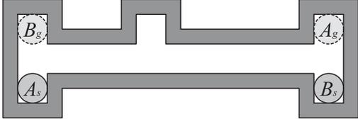
Fig. 2. An example scene in which the prioritization has a significant influence on the result. If robot  $A$  has priority over robot  $B$ , robot  $B$  can only start moving after  $A$  has reached its goal. If robot  $B$  has priority,  $A$  can use the cavity in the passageway to let robot  $B$  pass, giving a much better result.
