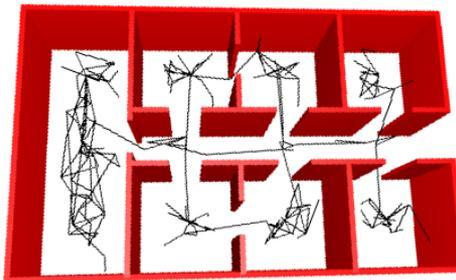
Fig. 10. A roadmap that is collision-free with respect to the static obstacles. The rotational degrees of freedom are not shown in the roadmap.
